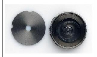
The complete mainspring exists of 3 accessories, here already put together. You can remove the cover with a little screwdriver and carefully remove the mainspring. Use Moebius 8300 for the mainspring and put it back in place (clockwise). Note the lug at the end of the mainspring. It should fall into the recess of both the barrel and cover.
