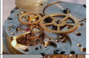
wheel bridge in place. Check continuously if the pivots of the wheels fall in the jewel holes correctly. Check if the gears run as they should and screw the bridge on the plate.
