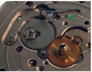
Put a little D5 where you see the 3 blue arrows. First put the hour wheel over Cannon pinion, then put the date indicator driving wheels (big and small) in place.
