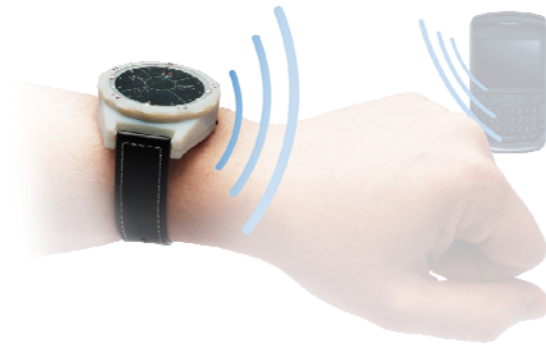
Figure 1: The haptic wristwatch communicates with a mobile device through Bluetooth®.
