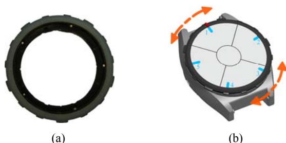
Figure 5: Bezel mechanism (a) with magnets shown. (b) When the tactile landmark (orange) on the bezel is aligned with one of the five mode indicators (blue), the bezel clicks into place.
